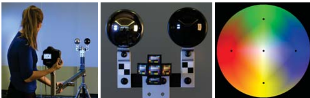
Figure 10: (a) Photographer using the fast multispectral lighting capture system (b) Image from the lighting capture camera with spheres and color charts. (c) Color-coded visualization of interpolating the five charts over the front hemisphere of surface normals.
