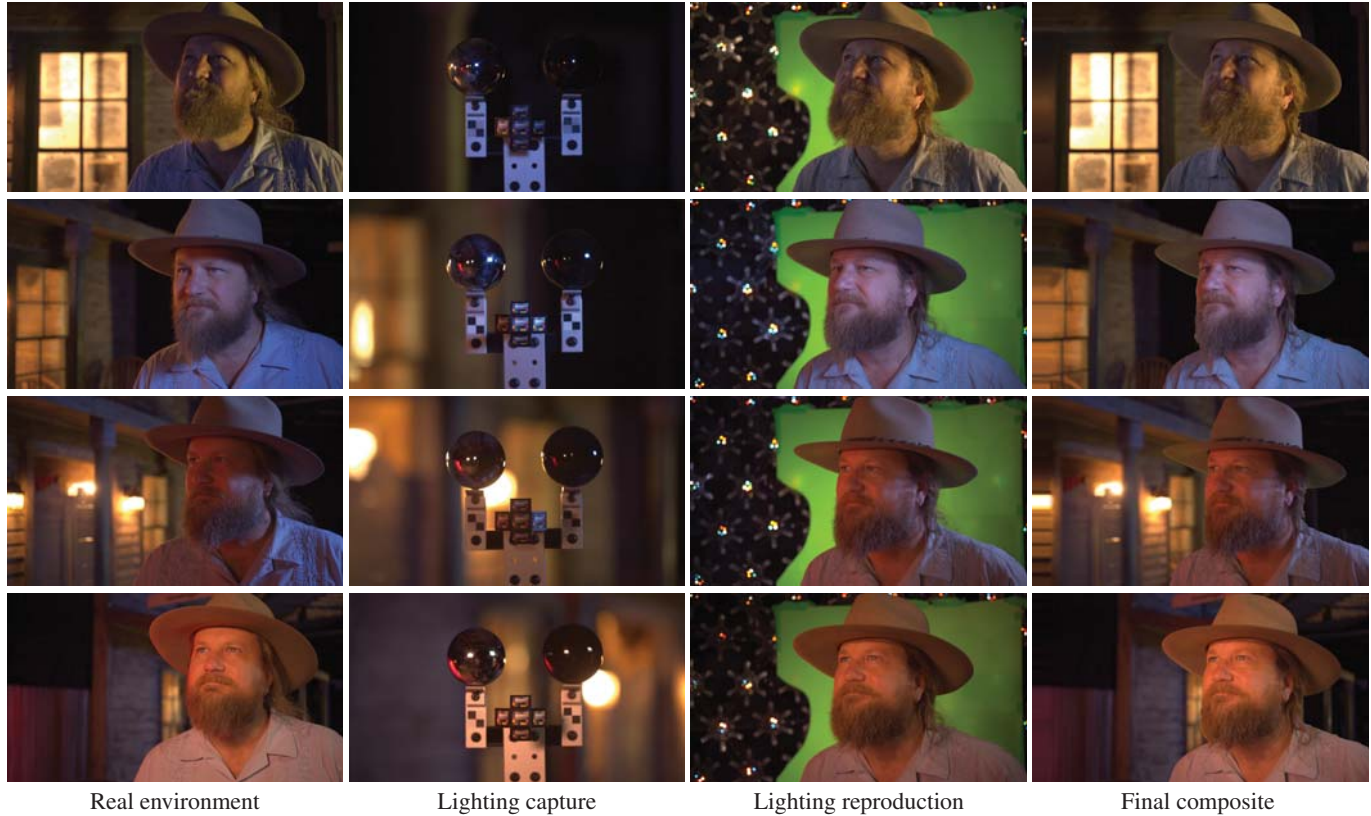
Figure 18: Frames from an image sequence where a subject moves through an environment, causing dynamic lighting from fluorescent, incandescent, and LED lights with various gels and diffusers. The last column composites the subject onto a clean plate of the set.
